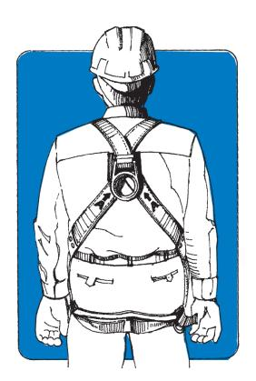
Hook on to the harness D-ring (marked "A") designed to arrest falls.
