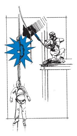
If you want to arrest a fall, your anchor must be capable of supporting at least 22 kN (5,000 lb.). Alternatively, when the potential arrest forces are known, an anchor that is capable of supporting the equivalent of two times the maximum arrest force generated by a falling worker is acceptable.
