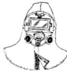
Class 7B Respirator facepiece for non-ionizing radiation protection
