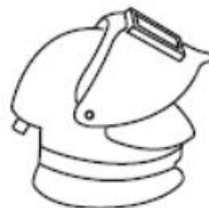
Class 7D Respirator facepiece with loose-fitting hood or helmet for non-ionizing radiation protection
