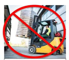
Always lower the load before a turn and raise the load only when necessary.
