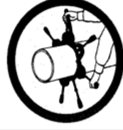
Cutting asbestos-containing pipe by hand.
